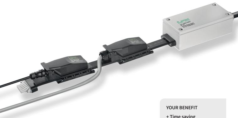
The podis® power bus system is ideal for decentralized power distribution in machines and systems with large dimensions. The power bus portfolio has now been extended to include a new variant for high currents. Significantly higher loads can now be supplied on a flat cable section. This means that the main distribution for a conveyor line, for example, can be installed very easily. Supply lines and
